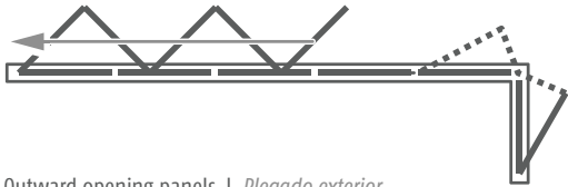
Outward opening panels | Plegado exterior
