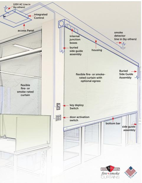
Fail Safe Features. This system is a gravity fail safe system. The M2500 features a fault report to indicate that the system requires a corrective action and the state of curtain deployment.
