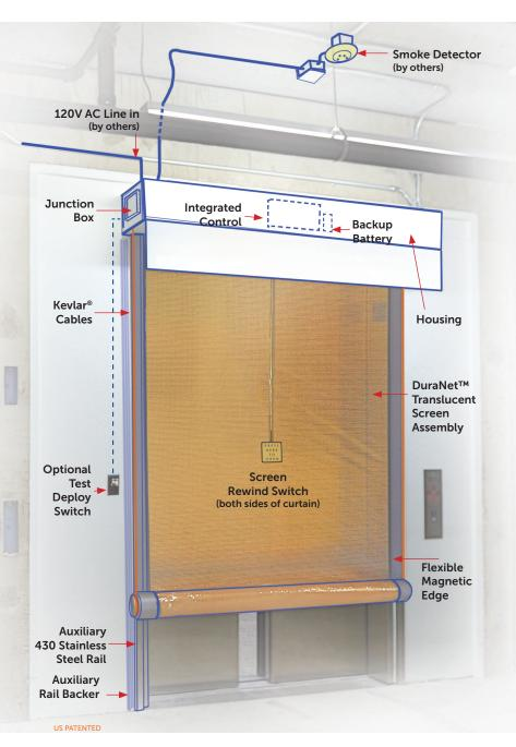
**Releasing Device.** Contained within the unit housing the **M600** control is tested in accordance with the UL 864 standard by Intertek Laboratories.
