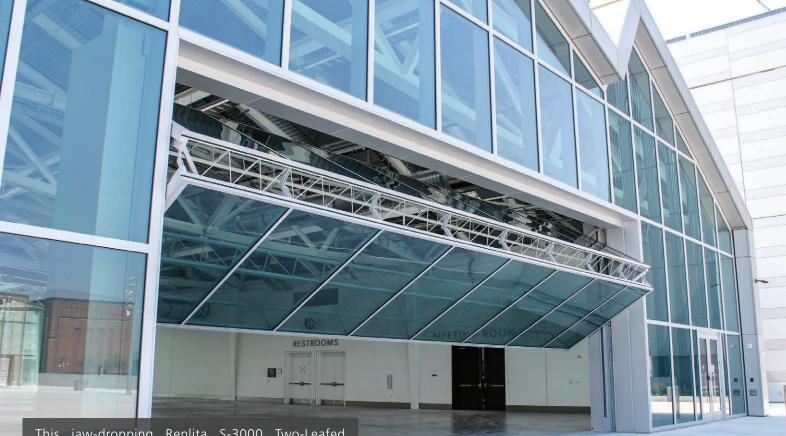
This jaw-dropping Renlita S-3000 Two-Leafed Overhead Foldaway/Bifold door at Jacob K. Javits Convention Center measures 41' wide x 17' tall and weighs over 9,000 lbs.
