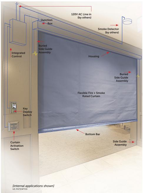
**Fail Safe Features.** The M2100 is a gravity fail safe system. The M2100 also features a fault report to indicate that the system requires a corrective action. The control unit monitors the state of curtain deployment.
