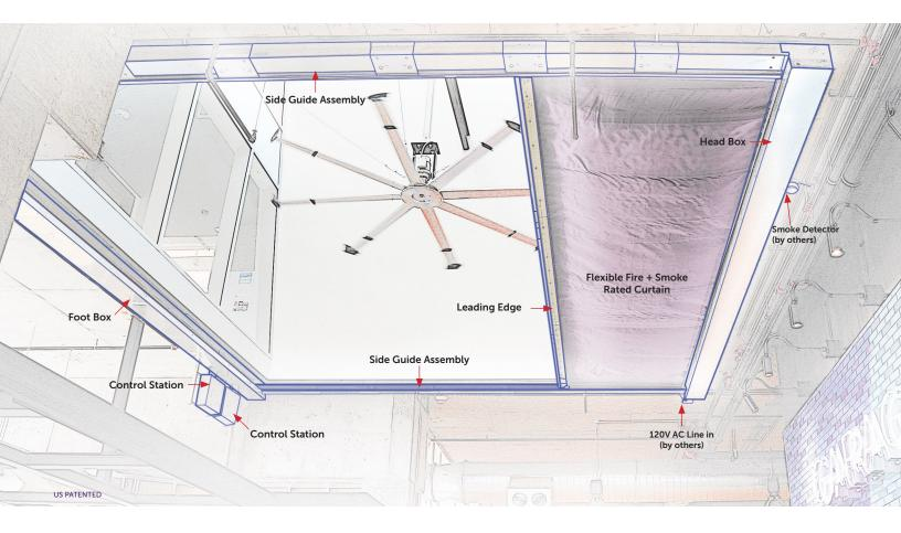
**System Operation.** The system is deployed upon a signal from the local smoke detection system or a smoke control panel. System power requirement is 120-volt AC. The unit is also equipped with a 24-volt DC battery back-up system that is maintained by the electronic controls. When required the system can also be connected to building standby power. The controls include a universal power supply that supports 230/240-volt operation.
