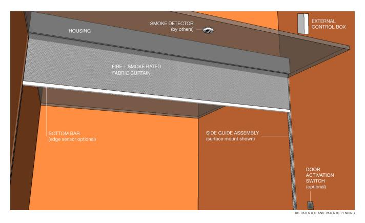
**Fail Safe Features.** The M2500 Egress is a gravity fail safe system. The M2500 Egress also features a fault report to indicate that the system requires a corrective action. This control also monitors the state of curtain deployment. An optional bottom bar sensing edge may be mounted to the curtain to guard against obstructions during deployment.
