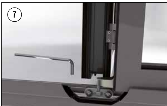
Post installation height adjustments possible on running mechanisms, in case of structure settling
