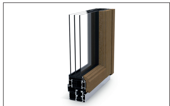
The ultra insulated aluminum folding door SF 75c offers optimum stability, burglar resistance as well as high operating tightness. The SF 75c is suitable for different applications such as balcony glazings or patio doors.
