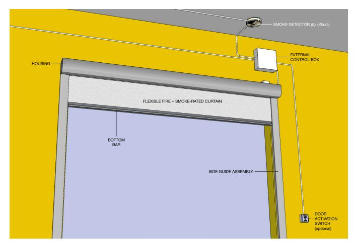
**Fail Safe Features.** The M2100|FS is a gravity fail safe system. The M2100|FS also features a fault report to indicate that the system requires a corrective action. The control unit monitors the state of curtain deployment.
