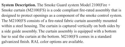
**Codes and Standards.** M2100|FS fulfills IBC requirements to provide an opening protective, where these assemblies are permitted as passive barriers used in conjunction with smoke control systems. This fire + smoke-rated curtain system can serve as opening protective for counter tops, openings in walls, and certain applications in atrium construction.
